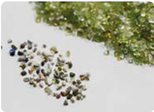
An example of a bad quality of crystal: impurities separated from the sample
